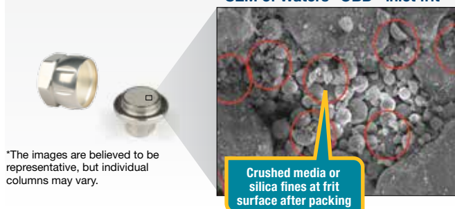
*SEM of Waters® OBD™ inlet frit
