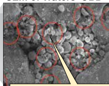
Crushed media or silica fines at frit surface after packing
